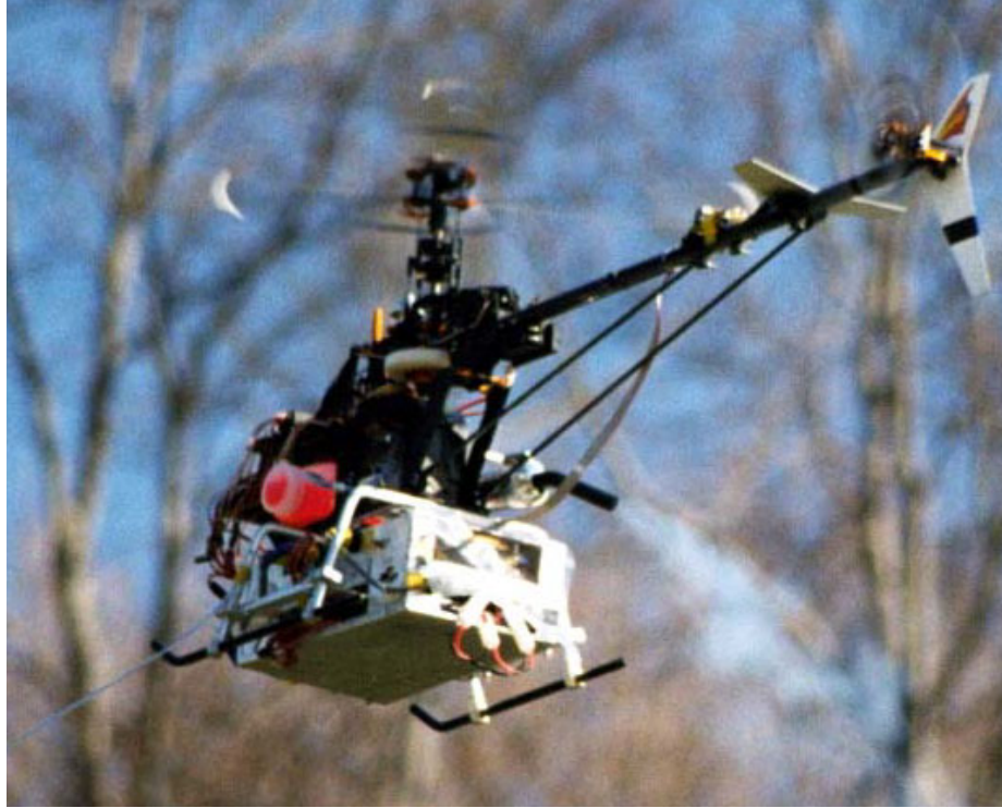
Figure 5.2: Close-up of instrumented X-Cell-90 helicopter in flight. The silver box between the helicopter's landing gear is the avionics box containing the flight computer, communication equipment, GPS, IMU and barometric altimeter. [photo courtesy of Vlad Gavrillets [58]].
