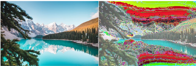
Fig. 2. Data corruption in crossbar-based OPCM memory from [13] due to crosstalk; (left) original image; (right) image after 4 writes to adjoining rows.
